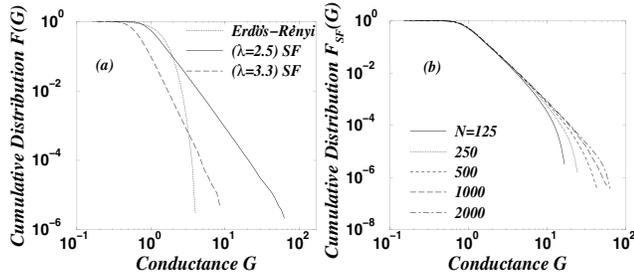
FIG. 1. (a) Comparison for networks with  $N = 8000$  nodes between the cumulative distribution functions for the Erdős-Rényi and the scale-free cases (with  $\lambda = 2.5$  and  $3.3$ ). Each curve represents the cumulative distribution  $F(G)$  vs  $G$ . The simulations have at least  $10^6$  realizations. (b) Effect of system size on  $F_{SF}(G)$  vs  $G$  for the case  $\lambda = 2.5$ . The cutoff value of the maximum conductance  $G_{max}$  progressively increases as  $N$  increases.
